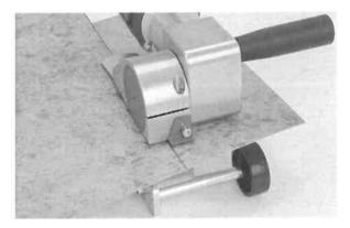
Should the tool stop while cutting, go into reverse and move the tool carefully towards the beginning of the cut. Never spin the wheels, or the polyurethane coated aluminium rings will be damaged.
