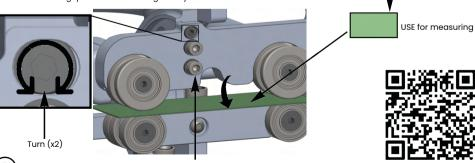
Tighten bolts with 5 mm allen key and test with workpiece
